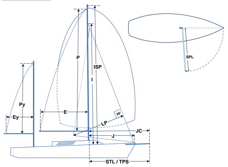
Dimension measured from the sheer line at the mast to the maximum hoist of the jib/genoa.
