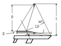
ISP: Height of the spinnaker halyard measured from deck sheer line abeam
